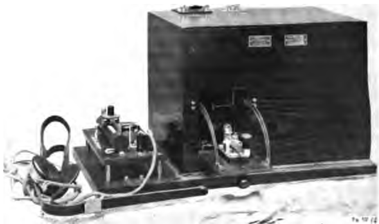
FIG. 169.—Small aeroplane installation.
